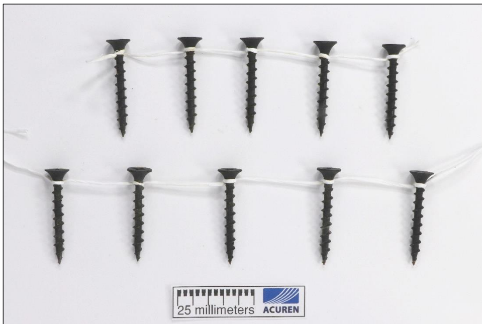
Figure 2 Black Phosphate 6 x 1- \frac{1}{4} Coarse Thread drywall screws after 48-hour exposure to salt fog.
